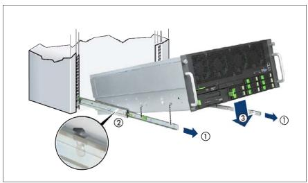
Figure 6: Inserting the server (a)
